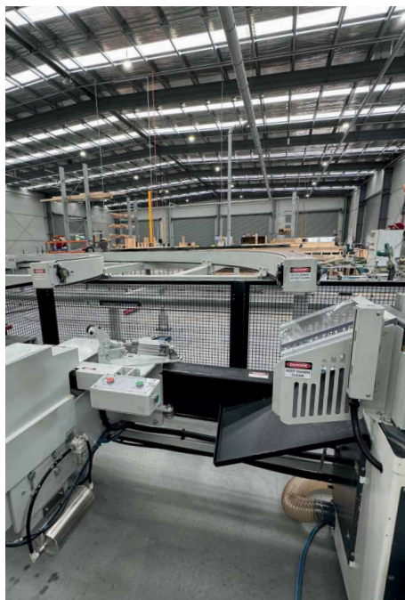
Above: Auto framing simplifies the process but can make both common and raked walls.
