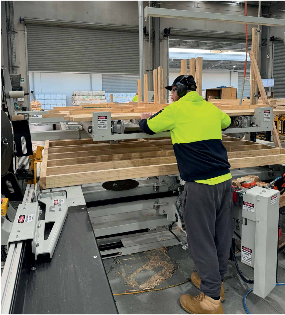
Above: The auto framer, where the top and bottom plates are nailed to the stud and noggin, to create the wall frame.
