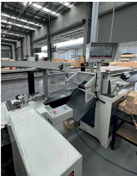
Above: Computerised nocking station which is fast and simple to operate.
