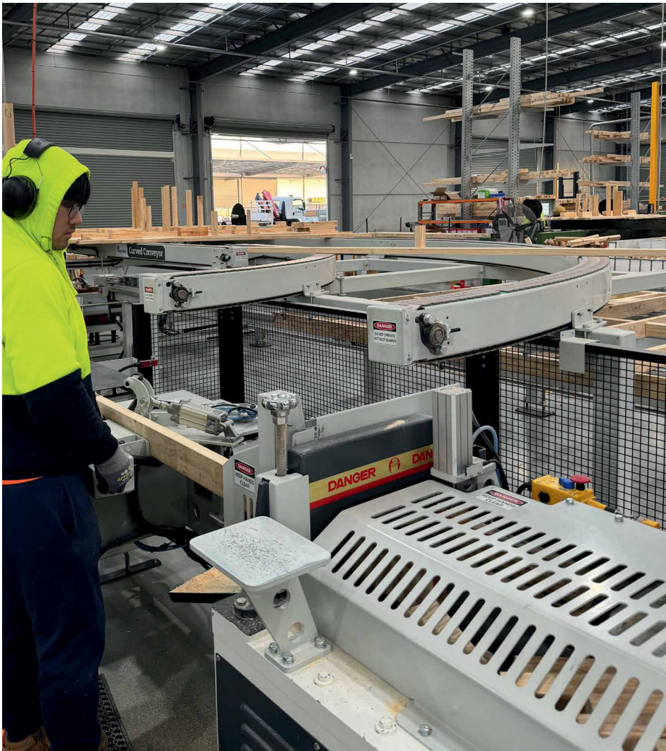
Above: This nocking station is where the noggins are cut to length and nailed to the studs.
