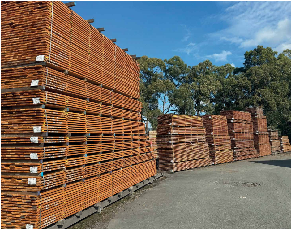
Above: Western Red Cedar, purchased green and put into sticker to dry naturally in the Australian climate.
