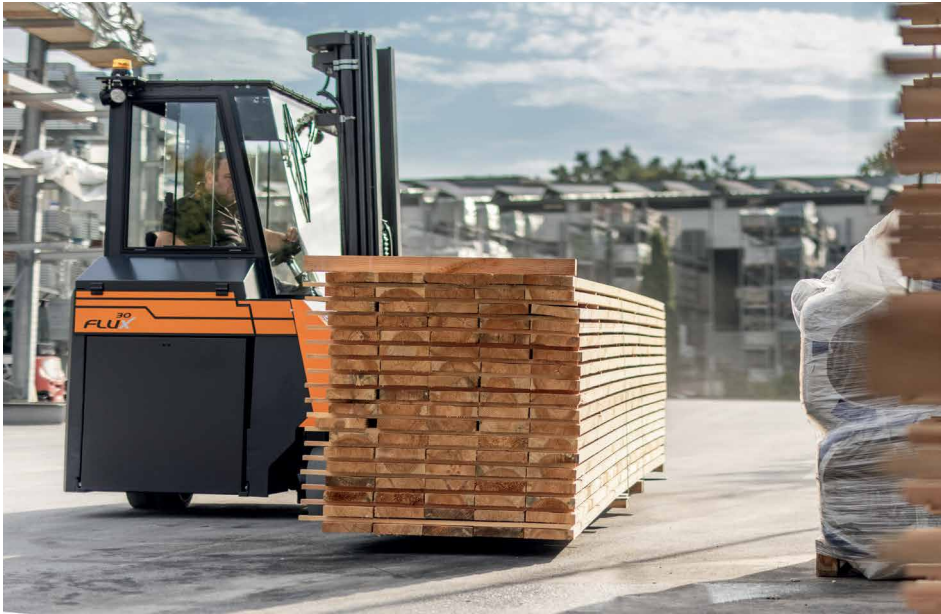
Left: The FluX Multidirectional Counterbalance Forklift, ideal for handling standard pallets and long loads.
