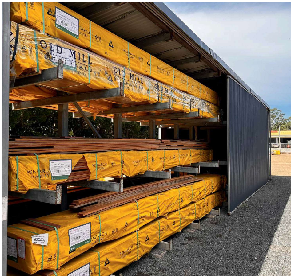
Above: When decking is delivered wrapped, keep it that way and off the ground until ready to install.
