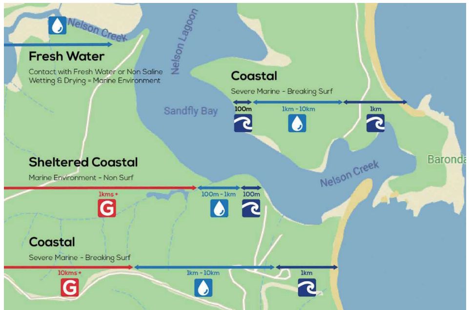
Above: A VUETRADE map showing which areas require stainless steel product (wave = 316, drop = 304).
