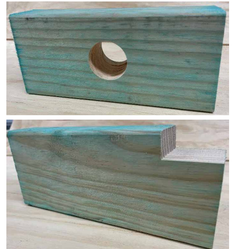
Above: Fig 2. Example of framing samples with a) notch, and b) drilled hole, exposed to Coptotermes acinaciformis in field trials.
