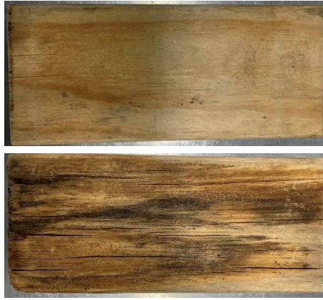
Above: Fig 3. Examples of Tanalith® Ti treated framing samples exposed to Coptotermes acinaciformis in a 39-week field trial, a) no decay present, and b) heavy decay present. Both specimens were resistant to attack by termites.
