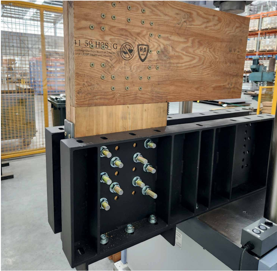
Above: Moment test of EcoBrace knee joint with LVL.
