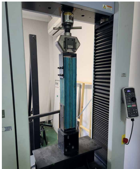
Above: Tensile test of EcoBrace column tie-down bracket.
