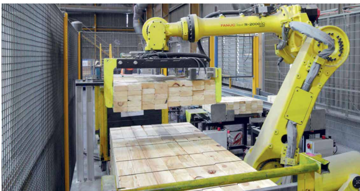
Above: Robot, Fanuc R-2000ic 165F in action, making light, speedy work of packing and strapping.
